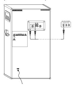
**Note:** If your audio source does not have AUX OUT R and L jacks, but has only a headphone or line out jack (such as on a portable tape or CD player), use a shielded Y-adapter cord with phono jacks on each end (such as Cat. No. 42-2475). Connect the single-plug end to the audio source's headphone or line out jack, and connect the other end's two phono plugs to the system's **AUX IN R** and **L** jacks.
